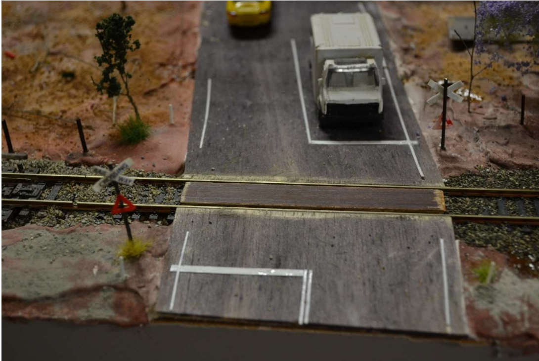
Above is an example of road markings around a railway level crossing. A guide post can be seen on the side of the road to the left.
