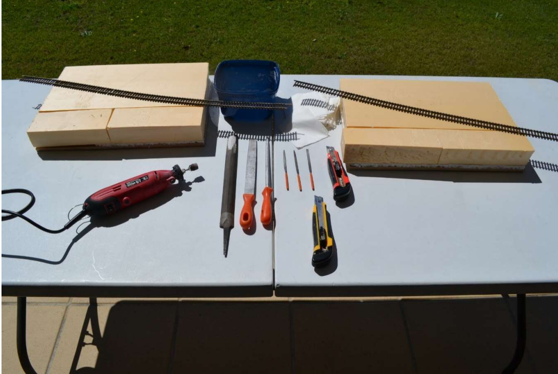
These are examples of high density foam and the tools needed to carve and contour them into the basic layers of scenery.
